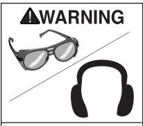
Operating this nailer can propel objects into the air, causing immediate eye damage. To protect yourself, always wear American National Standards Institute (ANSI) approved safety glasses or goggles when operating this equipment. In addition, this nailer discharges at approximately 85-90 decibels. To protect your hearing, always wear ANSI approved ear protection when operating.
